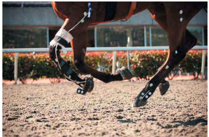
The horses were instrumented with an acceleration measurement package (a tri-axial piezoelectric-based accelerometer) and a force-measuring shoe (a dynamometric, force-measuring horseshoe). Acceleration and force signals were recorded using custom software.
