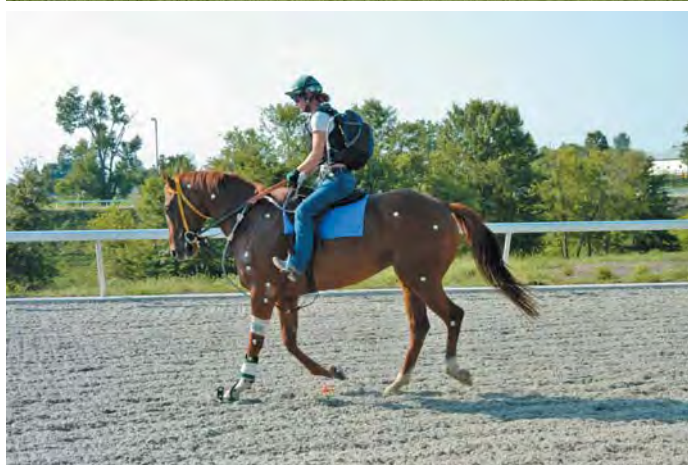
Hoof accelerations, ground reaction forces, and horse speed were measured on dirt (top photo), turf (middle photo), and synthetic (bottom photo) surfaces at the Keeneland Race Course, Lexington, Kentucky. Instrumented horses were walked, trotted, and cantered through the data collection corridor during three to four trials each of trot and canter.
