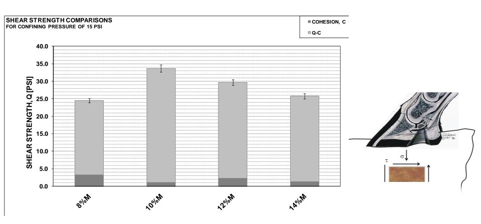
Moisture: 14% to 10% Shear Strength: 24.6 to 33.7 psi
