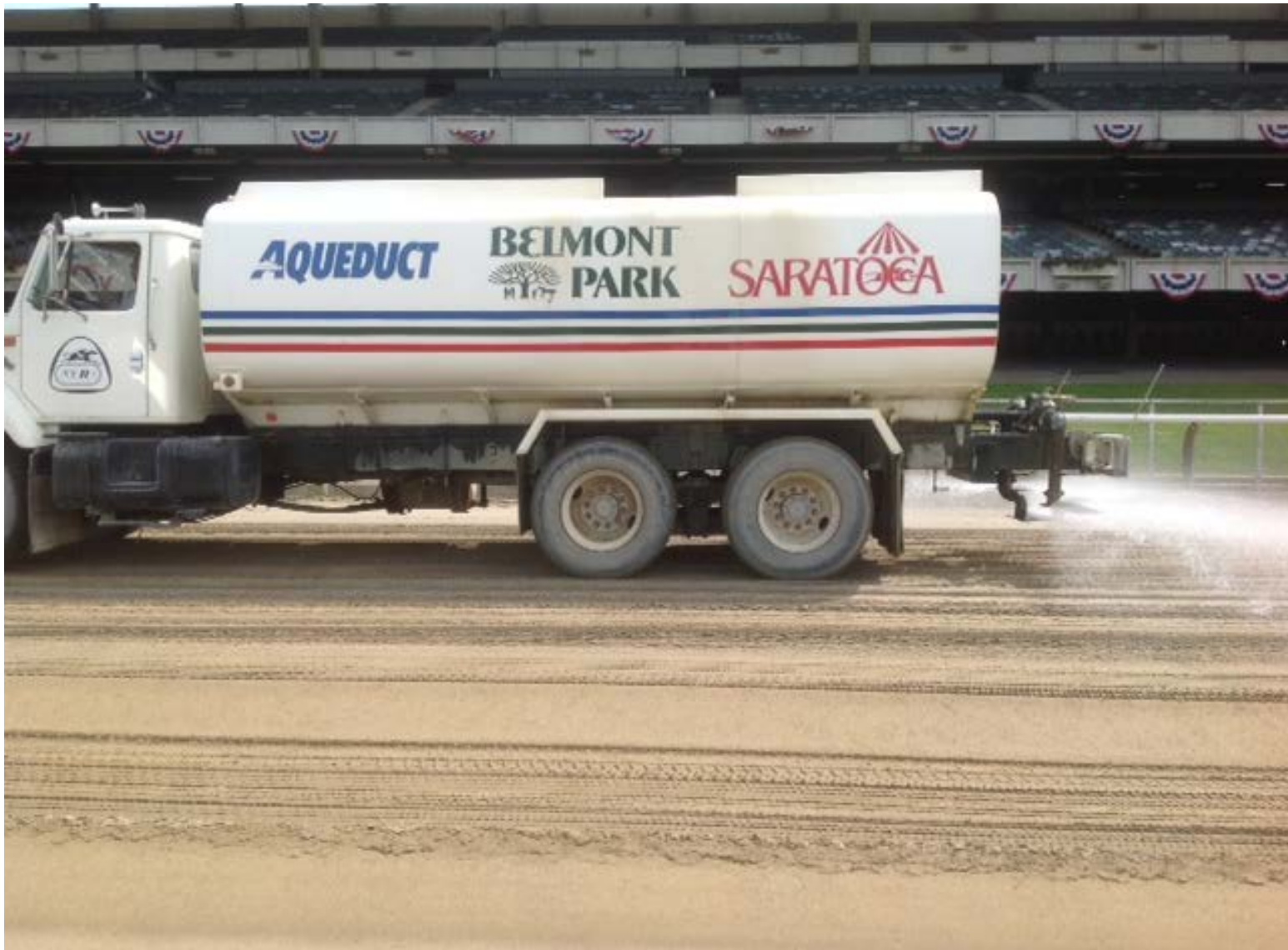
Flotation Tires, 4500 Gallon Tank, 3 spray patterns, used on outside of track and chutes
